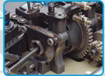
Braking system features bonded pads and machined steel rotors for maximum braking force and reduced fade
