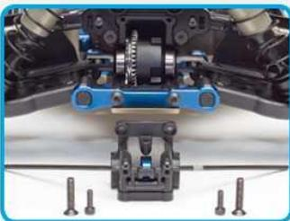
Gearboxes feature a 3.38:1 internal gear ratio with fast access differentials for quick removal, tuning and maintenance
