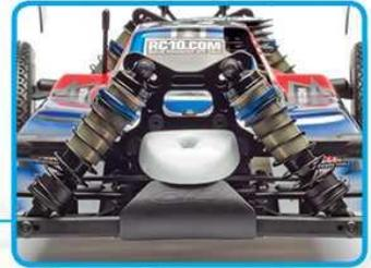
7075-T6 aluminum shock towers front and rear feature finely tuned shock mounting and upper arm positions
