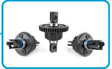
*42T ring and 12T pinion gears on front and rear differentials for improved gear ratios*
