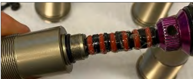
3. Insert assembly into shock body
