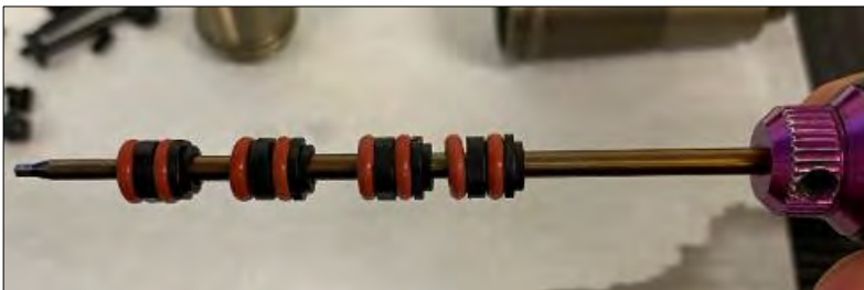
1. Orient bushing and O-rings onto shaft
