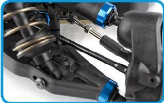
94mm CVA driveshafts increase traction and chassis support
