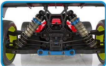
16mm Big Bore 6061 aluminum shock bodies and bleeder-style caps, with new 20mm I.D. springs
