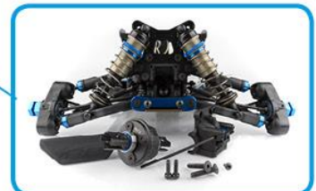
Easily accessible front and rear differentials
