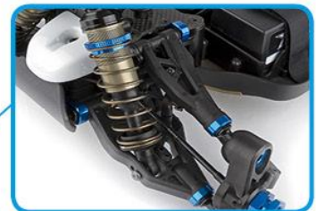
Suspension arms have been updated to modern race specs
