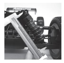
**Step 3:** Measure from the center of the shock standoff screw to the center of the shock riser button to get your final droop setting. The front shocks should both be set at the same lenght, as should the rear shocks. \* The normal droop setting is between 0-5mm from the FULL DROOP measurement.
