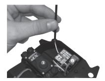
Note: route your receiver's antenna wire through the slot in the radio tray, and through your antenna tube.
