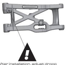
After installation, adjust droop screw to get a rear shock length of 122mm measured center to center on the shock cap / shock mount pin.
