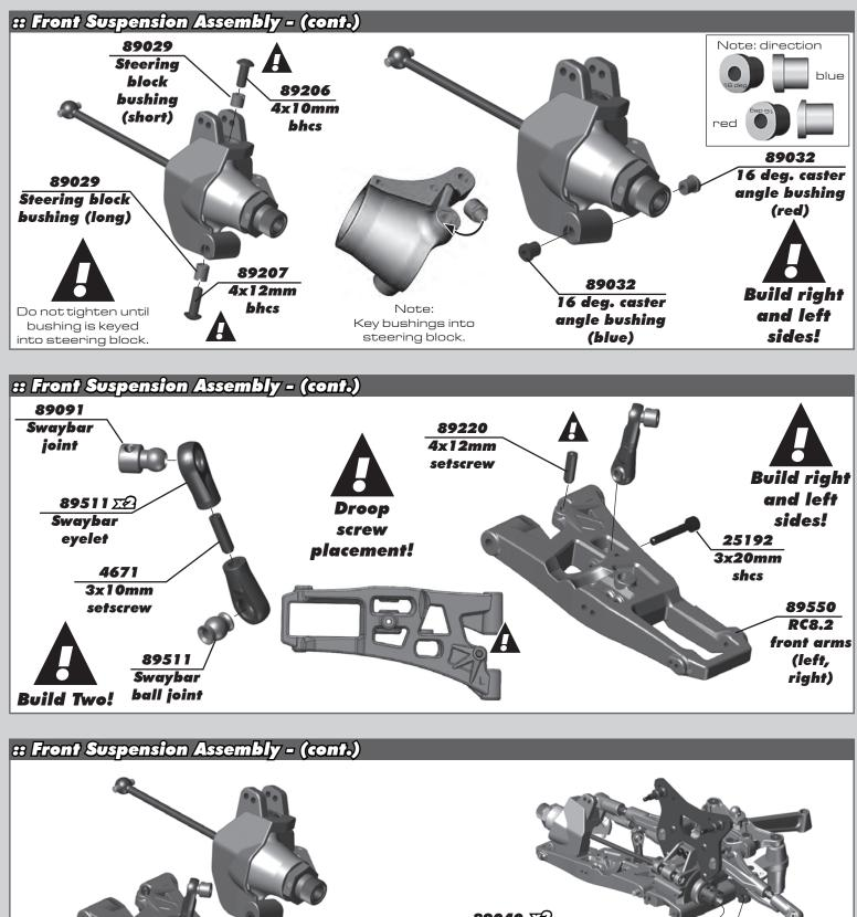
89041 Outer hinge pin 31520 2.5x6mm bhcs 89040 E
