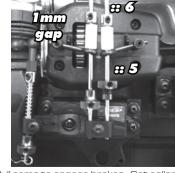
::5 - Pull cams to engage brakes. Set collar (with brakes engaged) to have 1mm gap between tubing and collar.
