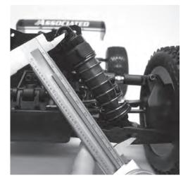
**Step 3:** Measure from the center of the shock standoff screw to the center of the shock riser button to get your final droop setting. The front shocks should both be set at the same lenght, as should the rear shocks. \* The normal droop setting is between O-5mm from the FULL DROOP measurement.
