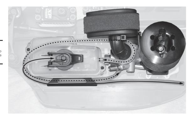
Pressure line from fuel tank lid to exhaust pipe nipple
