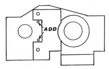
Photo #43 - Install both brake pins in the R bulkhead. Slip one of the #5238 brake shoes on the pins. Drill 2 #43 holes in the bulkhead in the position shown above. Tap the 2 holes for 4/40 threads, but only 2 threads deep. Do not tap all the way through. Remove brake shoe. Install both large ball bearings in both bulkheads.
