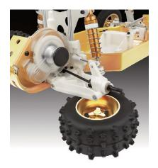
**Independent suspension with coil-over shocks** help smooth out the bumps. Precision molded nylon suspension components can be easily custom color dyed. A-Arm/Ball joint design permits static camber, camber rise, caster, ride height and spring rate tuning to suit every type of track.
