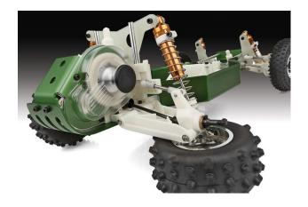
Independent suspension with coil-over shocks help smooth out the bumps. Precision molded nylon suspension components can be easily custom color dyed. A-Arm/Ball joint design permits static camber, camber rise, caster, ride height and spring rate tuning to suit every type of track.
