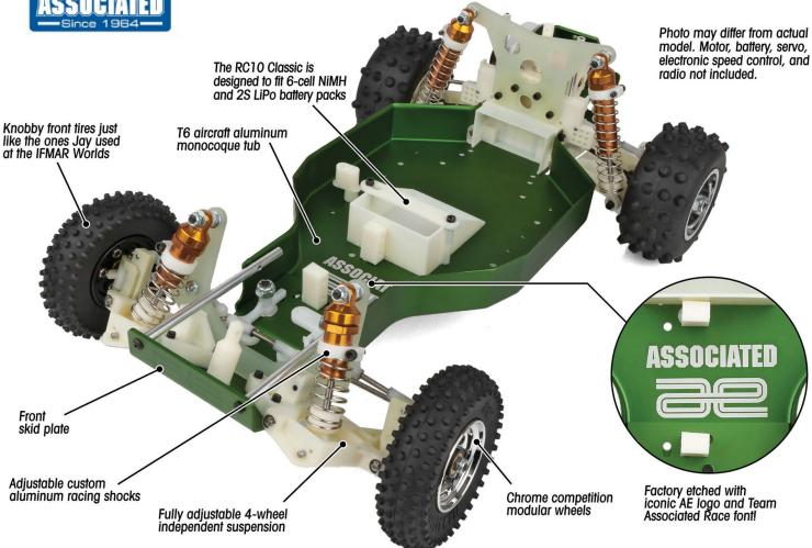
Rugged, yet light, the suspension gives you all the adjustability of full-size race buggies. The A-arm/Ball joint design allows precise camber, caster, ride height, and spring rate tuning. Even the adjustable VariLok differential is included, and the updated chassis fits 6-cell NiMh and 2S LiPo battery packs. Exceptional ground clearance and low center of gravity also contribute to the superb balance and performance of the RC10 over all types of terrain.
