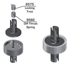
As you tighten the diff bolt, you will notice the T-nut ears moving closer to the bottom of the outdrive slot. This compresses the spring behind the T-nut. The spring should be completely
