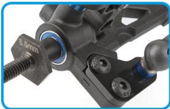
Bolt-on steering block arms for easy Ackermann adjustments
