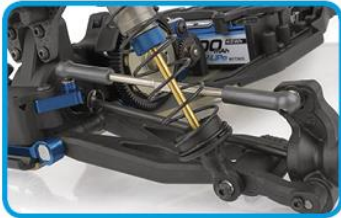
Heavy-duty rear axle with 91mm CVA bones
