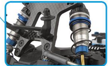
V2 12mm Big Bore threaded aluminum shocks with 3mm shafts and X-rings for improved smoothness
