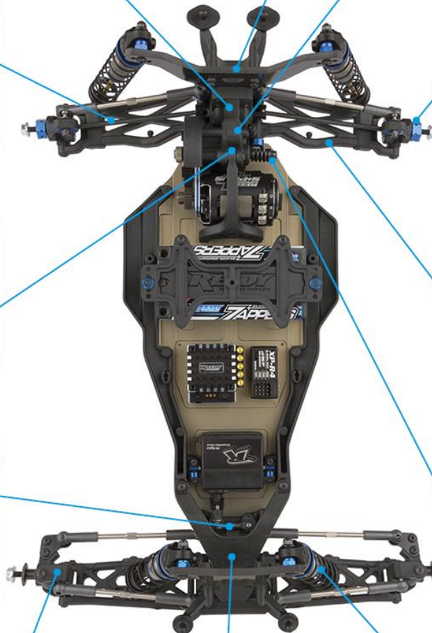
Heavy-duty rear axle with 91mm CVA bones
