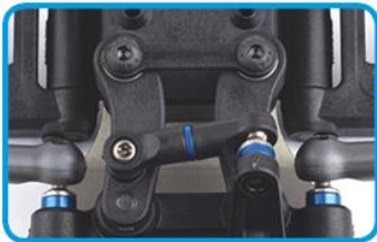
Reverse bellcrank steering allows more room for mounting electronics
