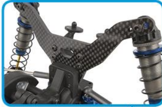
Heavy-duty routed graphite shock towers
