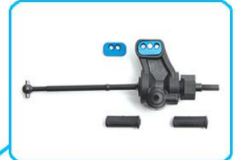
Rear hubs feature larger bearings and insert system to adjust camber link and toe-in
