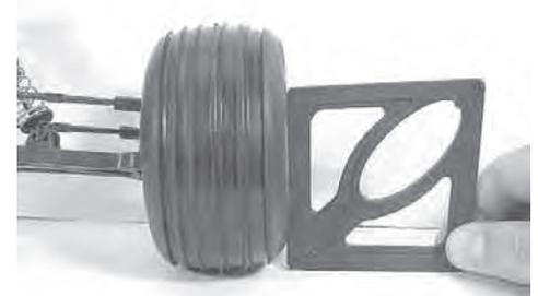
*Testing camber with the camber gauge*
