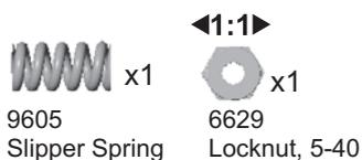
*Install locknut until even with end of shaft. Then tighten 3 turns for kit slipper setting. Recheck after initial run.*
