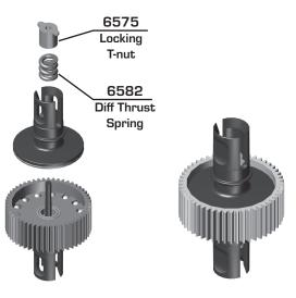
As you tighten the diff bolt, you will notice the T-nut ears moving closer to the bottom of the outdrive slot. This compresses the spring behind the T-nut. The spring should be completely
