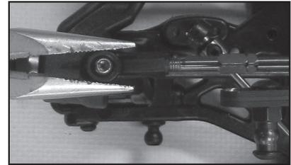
*It is important that the turnbuckle eyelets move freely once snapped on to the ballstud. If the fit is too tight, the car handling will be inconsistent. To check, grab turnbuckle eyelet with fingers and rotate the cup. If there is resistance, lightly squeeze ball cup with needle nose pliers as shown and test again. It is important that the ball cup be snapped onto the ballstud before squeezing with needle nose pliers. Be sure to check and adjust the fit for each ball cup that is installed.*
