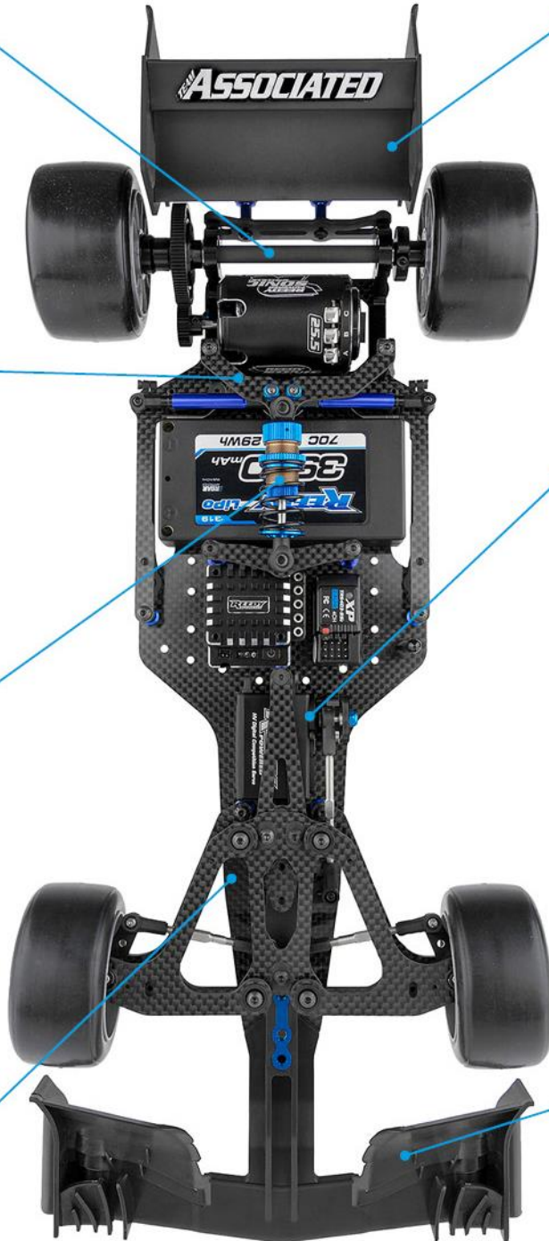
Rear wing with integrated 5mm mounting hole for option #29276 XP F6 Red LED Tail Light
