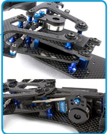
Two steering bellcrank options for fine tuning Ackermann and steering rate
