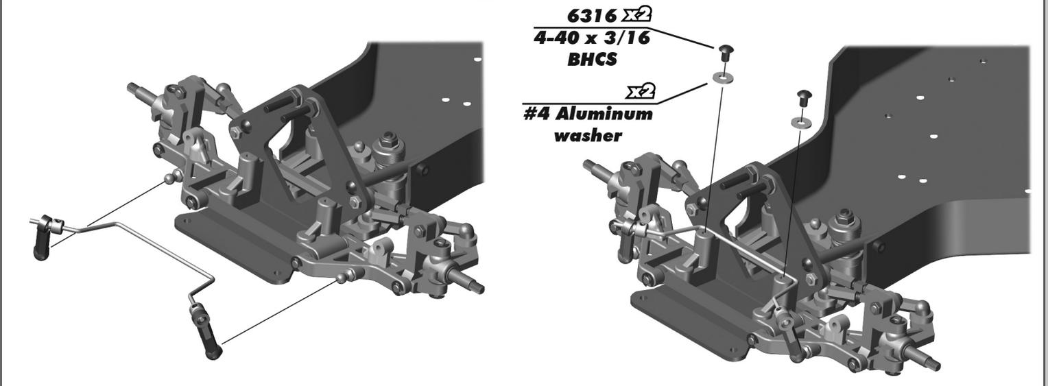
**:: Front Anti-Roll Bar / Bumper Build - Bag B - Step 3**
