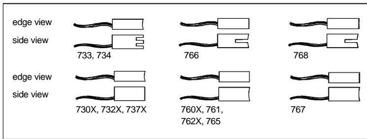
**MODIFIED MOTOR BRUSHES AND SPRINGS for standard commutator motors**
