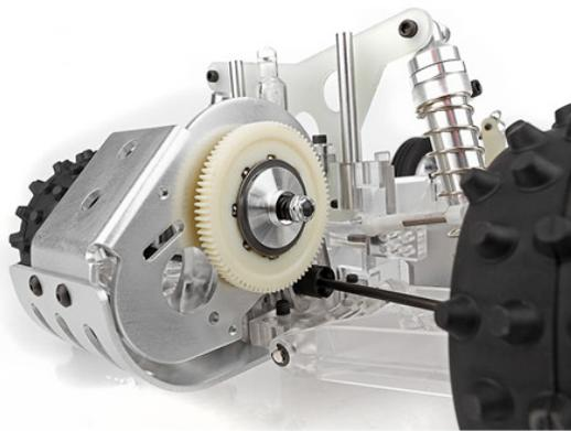
Full race rear suspension includes durable dogbone and stub axle drivetrain with pinned modular wheels. Quick-release knockoff design provides fast, accurate alignment. Low-profile gearbox uses VariLok adjustable diff and is protected by an integrated motor/heatsink.
