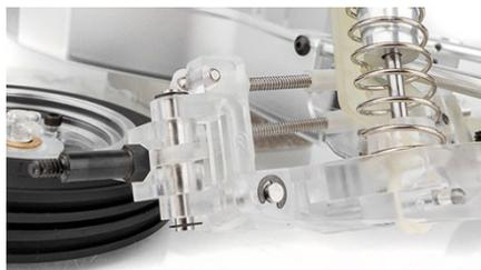
The RC10CC suspension gives you all the adjustability of full-size race buggies. The A-arm/Ball joint design allows precise camber, caster, ride height, and spring rate tuning. The adjustable VariLok differential is included, and the updated chassis fits 6-cell NiMH and 2S LiPo battery packs.
