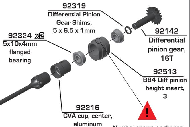
Number shown on the top and bottom of the rear insert after insertion should match the diff height desired.
