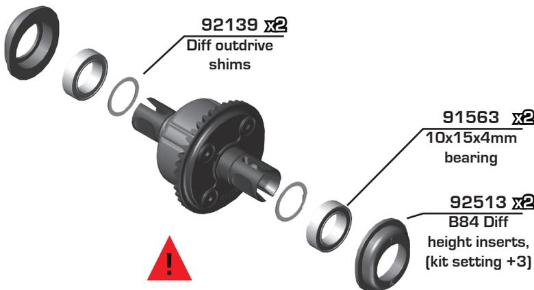
Start by shimming the diff with one shim on either side of the diff. If the diff is tight when inserted into the gearbox, remove one shim from the ring gear side and add it to the diff case side.
