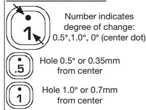
The aluminum front arm mounts utilize eccentric pill inserts to make fine adjustments to kick-up, pin height, and pin width. Adjustments can be made using the supplied inserts (#92014)
