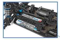
**Highly Adjustable Battery Holder with Thumb Tabs:** allows for easy battery removal and fine tuning of weight bias
