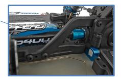
Chassis Bracing: fine tune chassis flex characteristics with upper and lower chassis bracing front and rear
