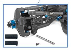
Insert adjustable caster block with 0, +/-1, and +/-2 degree inserts included
