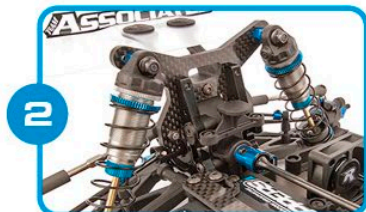
2 27.5mm V2 rear shock bodies with new 4mm carbon fiber shock tower that has been lowered by 5.5mm for maximum stability and predictability
