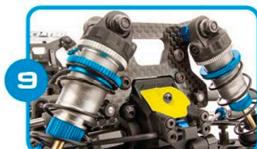
9 23mm shock bodies with new 4mm carbon fiber shock tower that has been lowered by 2mm and features an additional row of camber link positions
