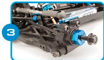
3 New rear arms and hub carriers with improved geometry and durability, combined with 66mm rear driveshafts and axles for more on-power traction and a predictable driving feeling
