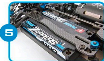
5 New 2.5mm carbon fiber battery strap has a simplified design with indexed battery locations, easier height setup, and battery removal for both standard and low-profile batteries
