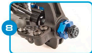
8 Updated 2.5mm carbon fiber steering arms for increased durability and 7075-T6 aluminum 9-degree caster blocks
