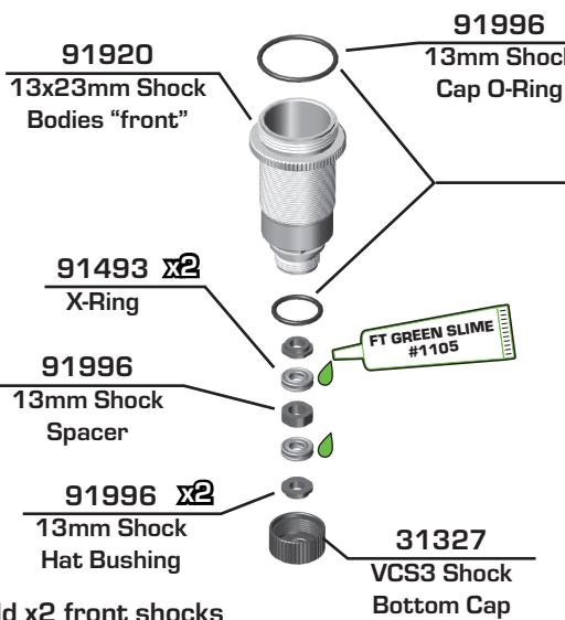
! Lightly rub shock oil on the O-ring before installation!
