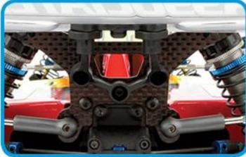
Stiff and lightweight 4mm thick carbon fiber shock towers
