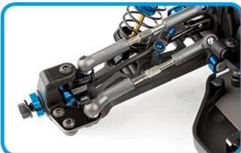
Robust suspension arms with multiple shock mounting positions
