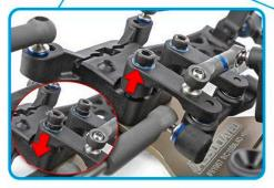
New adjustable height steering bellcrank and rack system for optimized bumpsteer at all ride heights and caster angles
