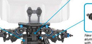
New 13mm big bore threaded aluminum shocks and springs with machined shock pistons and improved handling
