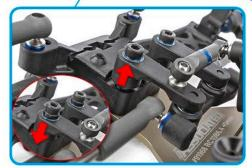
New adjustable height steering bellcrank and rack system for optimized bumpsteer at all ride heights and caster angles
