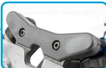
Updated carbon-fiber front and rear shock towers with new molded protective covers
