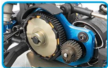
Octalock spur gear and 19mm Octalock LCF pads
