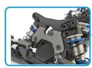
Heavy-duty V2 routed graphite front shock tower with tower guard
