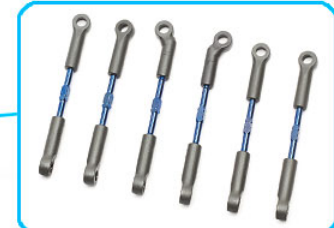
Heavy-duty lubricated ball cups and Factory Team titanium turnbuckles included
