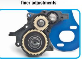
New transmission has stronger gears and a 14 carbide ball differential
