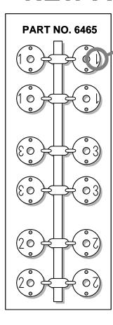
The shock pistons supplied are numbered #1, #2 and #3 so you can match them accurately to the shocks used on your kit according to the following tips:
