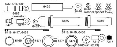
Associated's racing shocks have hard anodized and Teflon coated precision machined shock bodies for
