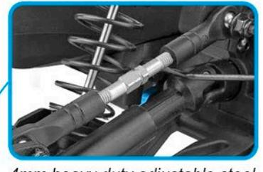
4mm heavy duty adjustable steel turnbuckles
