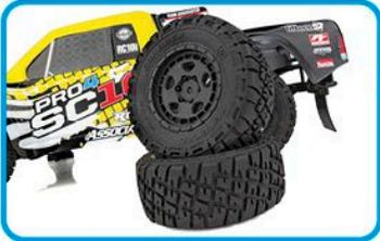
Fifteen52 Turbomac HD wheels equipped with high-grip General Tire GT® Grabber™ all-terrain tires
