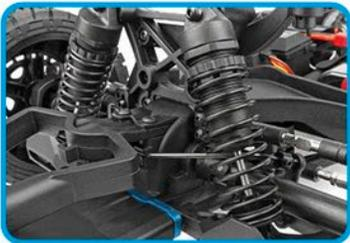
Threaded, oil-filled coil-over shock absorbers
