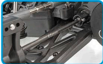
65mm rear CVA drive shafts for reliability
