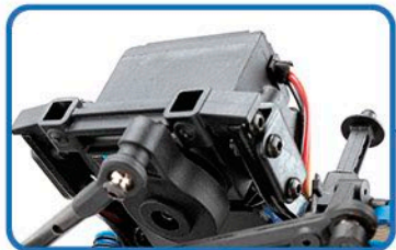
Chassis Mounted Steering (CMS) Servo
