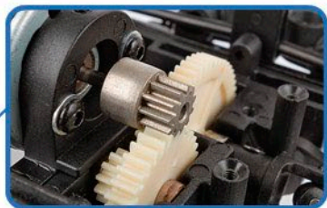
13.98:1 ratio 3-gear transmission with integrated motor mount
