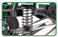
THREADED ALUMINUM SHOCK BODIES: Threaded aluminum and fluid-filled, these shocks keep the vehicle stable on the trail and retain fluid even in the roughest terrain.
