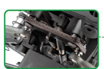
STEERING RACK: The included aluminum swing rack and steering plates give the IFS suspension a precise solid feel
