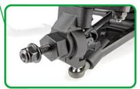
STEERING BLOCKS: 100% compatible with steering blocks from previous Enduro chassis and allows up to 45deg. of steering.
