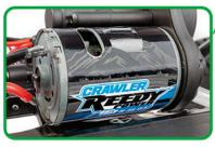
REEDY CRAWLER MOTOR: The Reedy 5-slot 16-turn brushed crawler motor provides ample torque with a smooth power delivery. This allows for slow precise acceleration while maintaining consistent power over rough terrain and obstacles.
