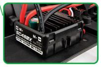
REEDY POWER ELECTRONIC SPEED CONTROLLER: The water-resistant SC480X brushed ESC is specifically programmed for crawling with proportional forward/reverse, dual auxiliary power output leads, LiPo low-voltage cutoff protections, and T-plug connector.
