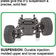
SUSPENSION: Durable injectionmolded upper and lower suspension arms with optimized ball cups provide maximum suspension articulation along with modern off-road vehicle suspension scale looks.
