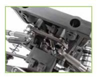
**STEERING RACK:** The included aluminum swing rack and steering plates give the IFS suspension a precise, solid feel.
