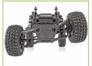
**SUSPENSION:** Injection molded upper and lower a-arms and optimized ball cups provide maximum suspension articulation.
