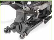
STEERING BLOCKS: 100% compatible with steering blocks from previous Enduro chassis and allows up to 45° of steering.
