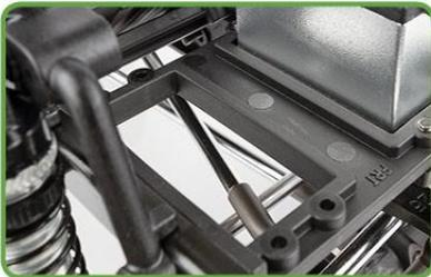
**Integrated servo winch mount:** Mounting a winch directly to the chassis is the strongest and most reliable spot. Positioned alongside the steering servo for overall chassis balance and weight distribution.
