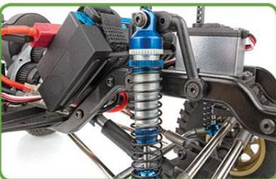
**Threaded Aluminum shock bodies:** 90mm threaded aluminum shocks keep the vehicle stable on the trail and retain oil even in the roughest terrain.
