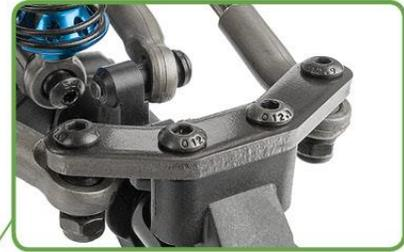
**Aluminum steering plates:** Bolt-on aluminum steering plates allow for more adjustment, strength, and future modification for the user.
