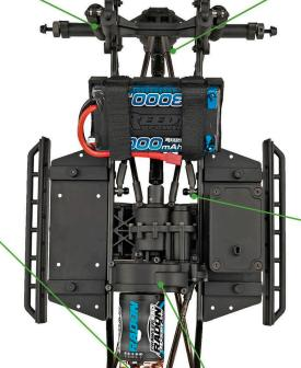
Steel Pivot Balls:30 Factory Team machined steel pivot balls are more durable and smoother than our previous plastic pivot balls. Providing a longer-lasting suspension.
