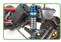
Threaded Aluminum shock bodies: 90mm threaded aluminum shocks keep the vehicle stable on the trail and retain oil even in the roughest terrain.
