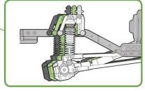
Adjustable wheelbase: The included 4-link bars provide the ability for the Enduro's wheelbase to be adjusted from 12.3, 12.0, and 11.8 inches. This allows for a wide variety of body styles to be used.
