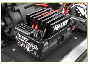
**REEDY POWER ELECTRONIC SPEED CONTROLLER (ESC):** The water resistant SC400X brushed ESC is specifically programmed for crawling with proportional forward/reverse, dual auxiliary power output leads, LiPo low-voltage cutoff protections, and T-plug connector.
