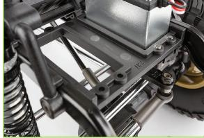
INTEGRATED SERVO WINCH MOUNT: Mounting a winch directly to the chassis is the strongest and most reliable spot on any trail rig. Positioned alongside the steering servo for overall chassis balance and weight distribution.
