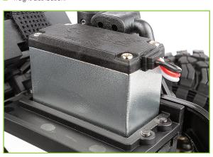
**RADIO & SERVO:** The XPI30, 2.4GHz, 3-channel radio and receiver together with a Reedy Power I320MG (metal gear) water resistant servo pushing out I73oz-in (I2.5kg-cm) of torque at 6V is the perfect setup for keeping the Enduro under control on the trail.
