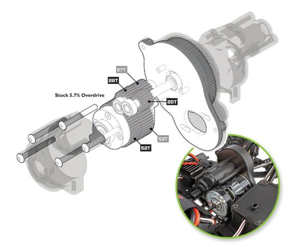
**STEALTH® X GEARBOX WITH ADJUSTABLE OVERDRIVE GEARS:** At the heart of the Enduro is our revolutionary Stealth® X gearbox. Although the exterior appears to have a conventional 3-gear transmission look, the inside is far from conventional. The Stealth® X features the ability to adjust the rear drive ratio independently from the front drive in 3 levels.
