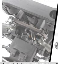
The included aluminum swing rack and steering plates give the IFS suspension a precise, solid feel.
