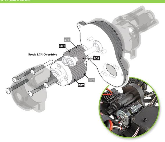
**STEALTH® X GEARBOX WITH ADJUSTABLE OVERDRIVE GEARS:** At the heart of the Enduro is our revolutionary Stealth® X gearbox. Although the exterior appears to have a conventional 3-gear transmission look, the inside is far from conventional. The Stealth® X features the ability to adjust the rear drive ratio independently from the front drive in 3 levels.
