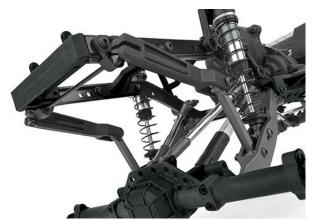
REAR ANTI-ROLL BAR: The rear anti-roll bar (above) helps keep the rear suspension stable while driving over rough terrain and improves climbability on steep inclines or side hills.
