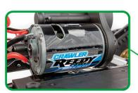
REEDY POWER CRAWLER MOTOR: The Reedy Power 5-slot 16-turn brushed crawler motor provides ample torque with a smooth power delivery. This allows for slow precise acceleration while maintaining consistent power over rough terrain and obstacles.
