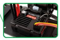
ELECTRONIC SPEED CON-TROLLER (ESC): The water resistant brushed ESC is specifically programmed for crawling with proportional forward/ reverse, dual auxiliary power output leads, LiPo low-voltage cutoff protections, and T-plug connector.
