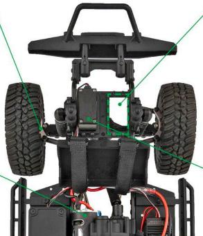
INTEGRATED SERVO WINCH MOUNT: Mounting a winch directly to the chassis is the strongest and most reliable spot on any trail rig. Positioned alongside the steering servo for overall chassis balance and weight distribution.
