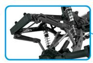
TRAILING ARM REAR SUS-PENSION: This design moves the shocks forward, thus improving weight bias. This allows for a larger window for shock tuning and an optimized anti-roll bar mounting position.
