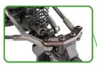
BTA steering & Aluminum steering plates: Behind-theaxle steering provides better approach angles, more clearance, and a cleaner look. Bolt-on aluminum steering plates allow for more adjustments, strength, and future modifications.
