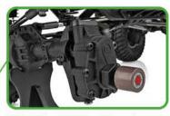
PORTAL AXLES: When it comes to rock crawling, ground clearance is crucial. That's why the Enduro Ecto Portal RTR includes our all-new high-clearance portal axles. With almost an inch of added center axle clearance, over standard straight axles, getting over tough obstacles is a breeze.
