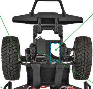
INTEGRATED SERVO WINCH MOUNT: Mounting a winch directly to the chassis is the strongest and most reliable spot on any trail rig. Positioned alongside the steering servo for overall chassis balance and weight distribution.
