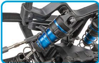
Aluminum 12mm big bore coil-over shock absorbers
