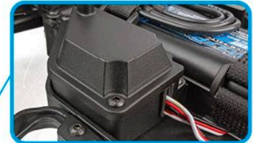
Water-resistant enclosed receiver box
